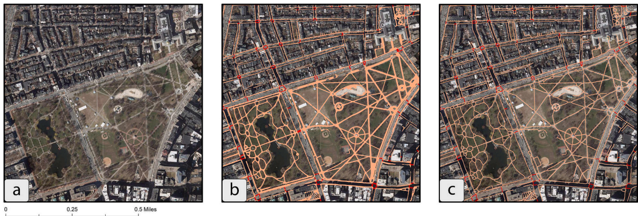
Fig. 4. Boston Commons: a) Aerial image, b) Detected sidewalk and footpath polygons (in orange) and detected crosswalks (in red), c) Fitted sidewalk, crosswalk, and footpath centerlines superimposed on the aerial image. (For interpretation of the references to color in this figure legend, the reader is referred to the web version of this article).
